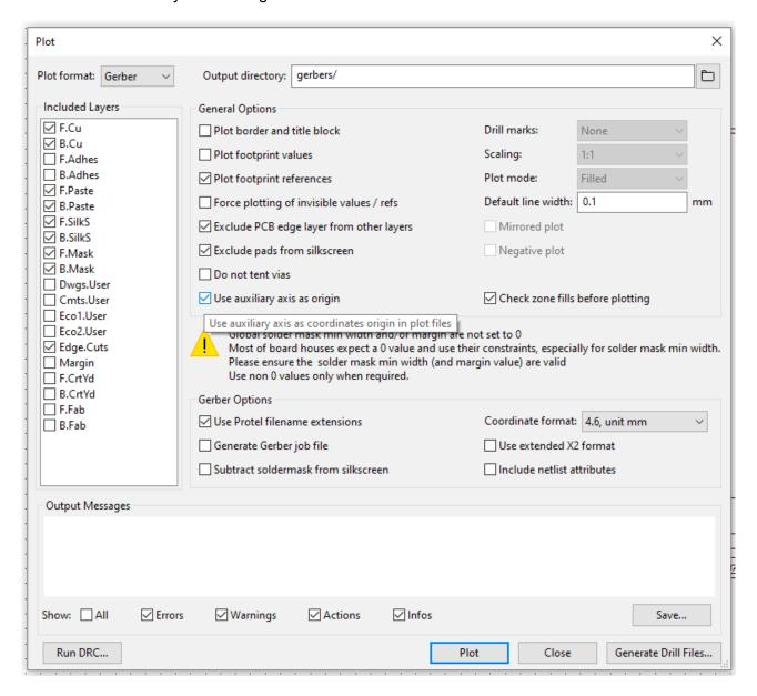
You can now proceed with generating the layout Gerbers by pressing the "Plot" button and Excellon drill files by pressing the "Generate Drill Files..." button. All CAM data will now be referenced to the Grid Origin that you defined and the design can be conveniently placed anywhere on your CNC table by using the machine's G-code driver's zero function.
