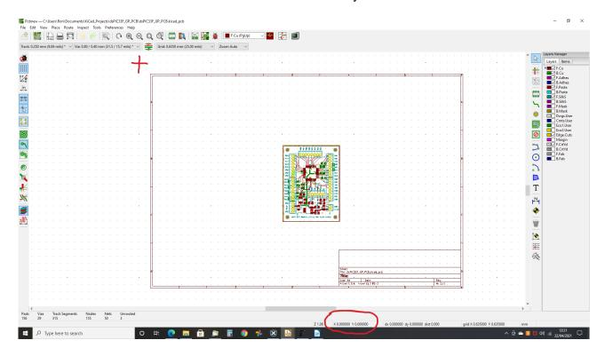
When you create the CAM files for your design, unless you tell KiCAD otherwise it will use this default origin as the reference for the design. When you generate G-code files for your CNC, (using a program such as FlatCAM), the G-code coordinates faithfully reflect the screen position of the design in Pcbnew. This may make your G-code data fall beyond the X-Y reach of your CNC
