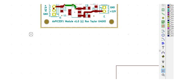
To change the position of the Grid Origin, select the Set Grid Origin Point and define a new point using the same process as above. The Grid Origin will be moved to this new point.
